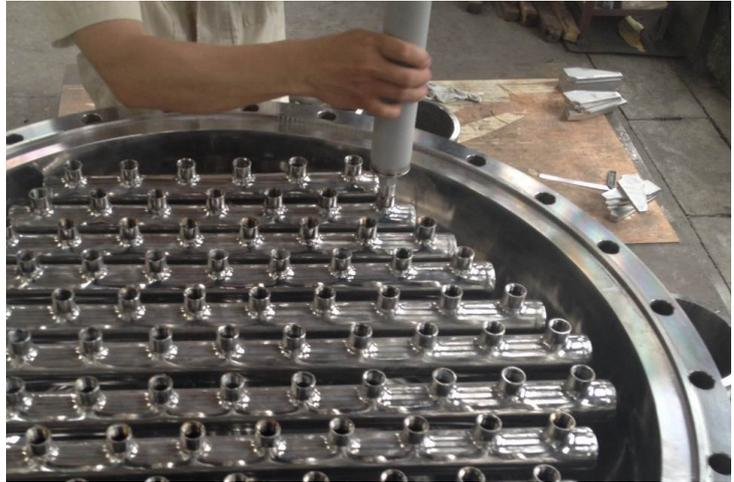
Additionally, when the feed solids concentration fluctuates significantly and larger quantities of solids are expected at certain moments the operating cost of cartridge filters (due to frequent replacement of elements) can quickly amount to considerable sums which may be better invested into a more sustainable solution. For such cases the sinter metal (SM) guard filter may present an interesting option.
